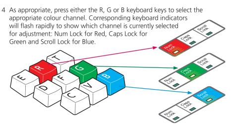
5 Press the  $\square$  and  $\square$  keys to retard or advance the timing of the selected colour channel respectively. On screen you will see a change in the position of the selected colour crosses in relation to the other two.
